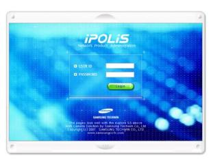
Use the IP address and port assigned to the product to access the Web Viewer Log-in page. The URL to access the page will be similar to http://192.168.1.100:4000. If the port value has been changed from the default value of 4000, use the changed value instead after the colons. Use the ID and password from SNM-128S and click "Login". The default ID and password are [admin] and [11111111] (eight ones). The password may be changed, but the ID may not.
